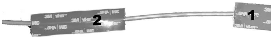
Figure 5: SolarSCADA Back of Module Temperature Sensor
